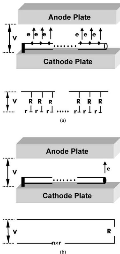
Fig. 11. Equivalent circuit model for field emission according to dominant emission mechanism (a) body-emission dominating case (b) tip-emission dominating case.
