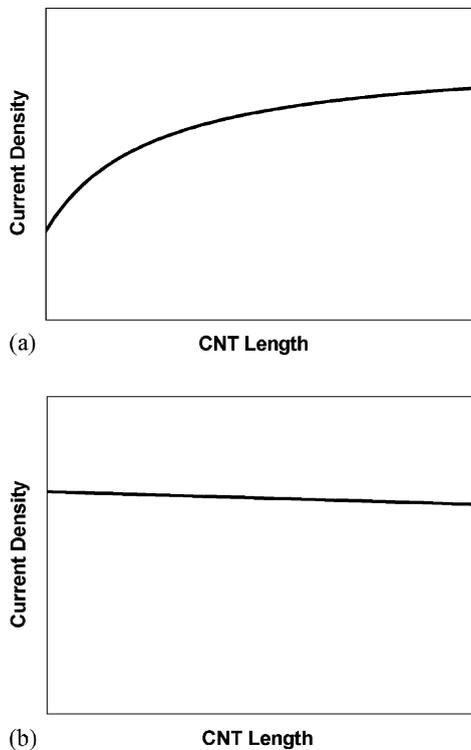
Fig. 12. Change in current density depending upon the length of a carbon nanotube in the case of two different emission mechanisms (a) body-emission dominating case (b) tip-emission dominating case.
