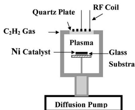
Fig. 1. Schematic diagram of TCP type rf plasma enhanced CVD system.
