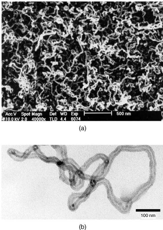
Fig. 3. (a) SEM and (b) TEM image of carbon nanotubes produced by rf PE-CVD.
