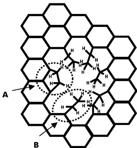
Fig. 8. Proposed surface structure of carbon nanotubes grown by rf PE-CVD.
