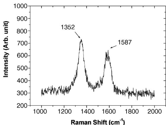
Fig. 4. Raman spectrum of carbon nanotubes synthesized by rf PE-CVD.
