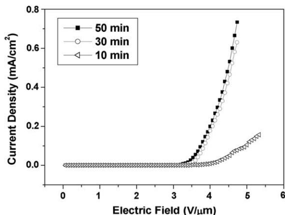
Fig. 9. Field emission curves depending upon carbon nanotube growth time.
