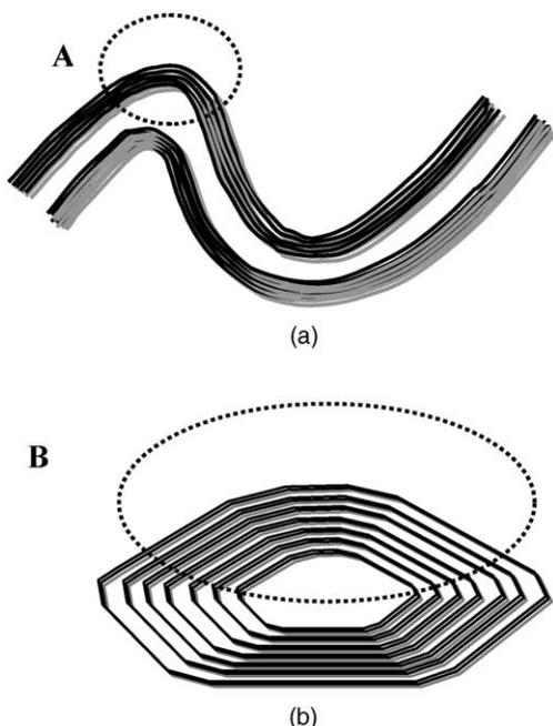
Fig. 5. Schematic diagram of (a) curved carbon nanotube and (b) carbon nanoparticle.
