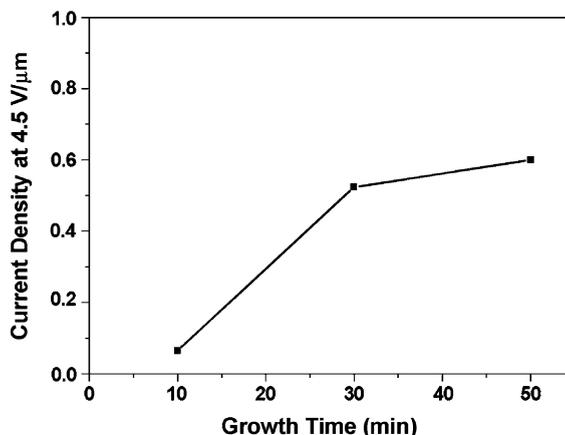
Fig. 10. Change in field emission current density depending upon carbon nanotubes growth time.
