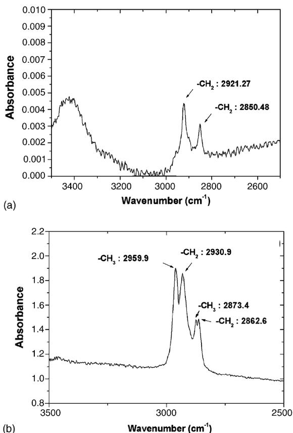
Fig. 6. FTIR spectra of carbon nanotubes produced by rf PE-CVD (a) arc-discharge (b) rf PE-CVD.
