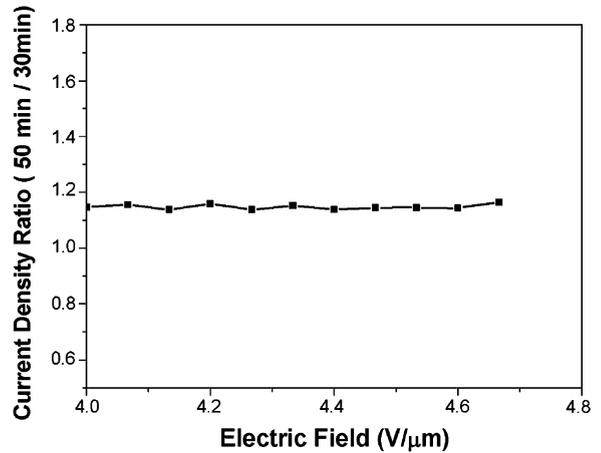
Fig. 13. Field emission current density ratio (50 min sample/30 min sample) as a function of electric field.
