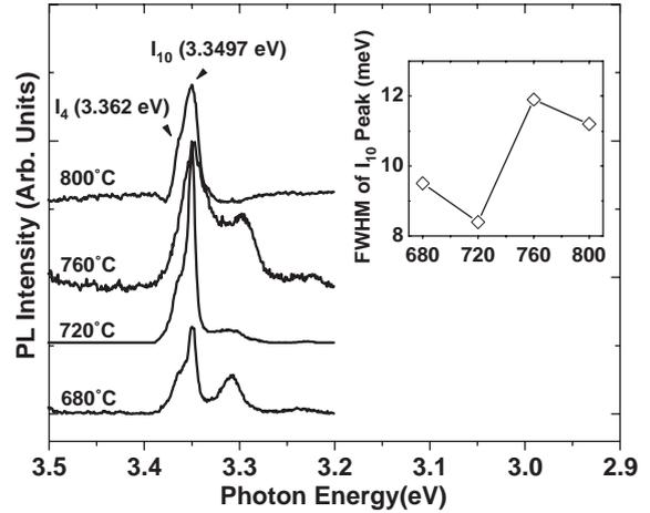
Fig. 5. Low-temperature (10 K) PL measurement results of the ZnO films on  $\text{Al}_2\text{O}_3$  (0001) substrates with different growth temperatures.
