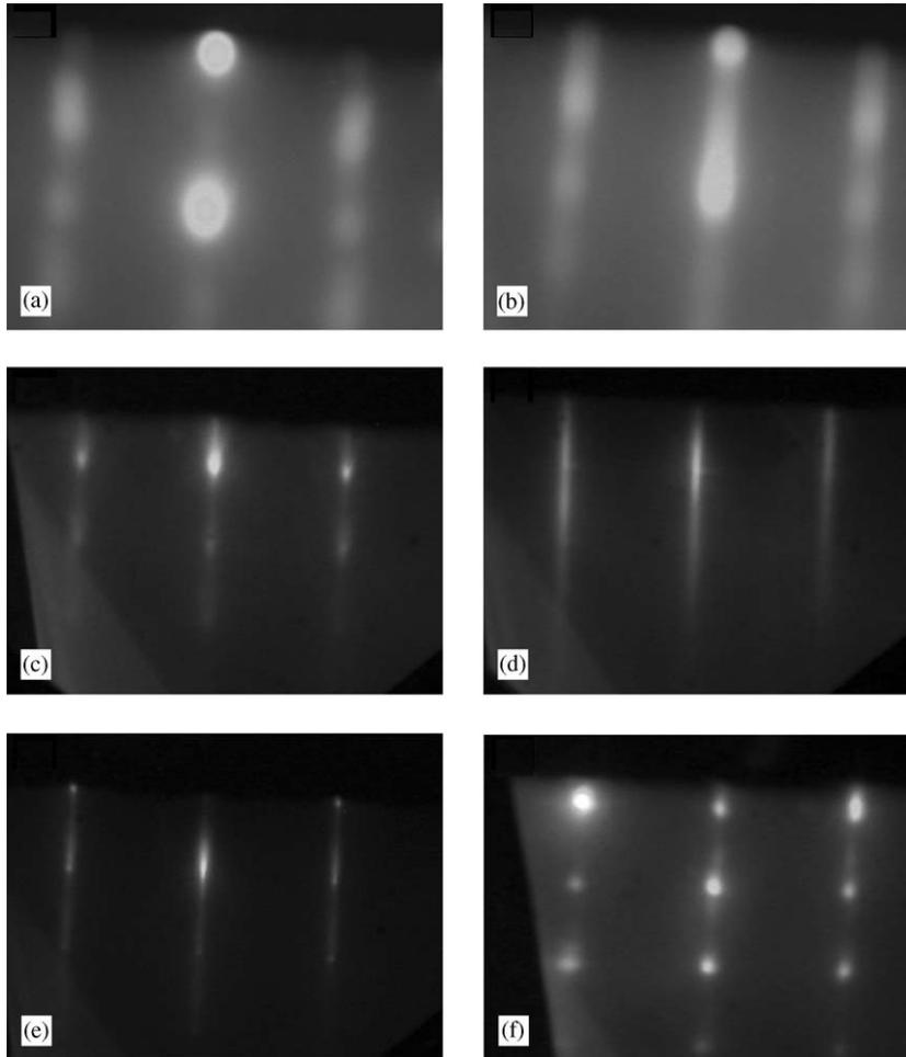
Fig. 1.  $\langle 1\bar{2}10 \rangle$  RHEED patterns of (a) LT-buffer layer 15 nm deposited at 500 °C and (b) after annealing the buffer layer for 30 min at 720 °C. Subsequent deposition of HT-ZnO at (c) 680, (d) 720, (e) 760, and (f) 800 °C.
