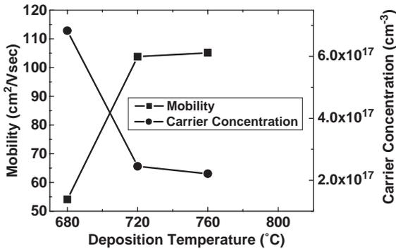
Fig. 4. Hall measurement results of the ZnO films deposited with on  $\text{Al}_2\text{O}_3$  (0001) substrates with different growth temperatures.
