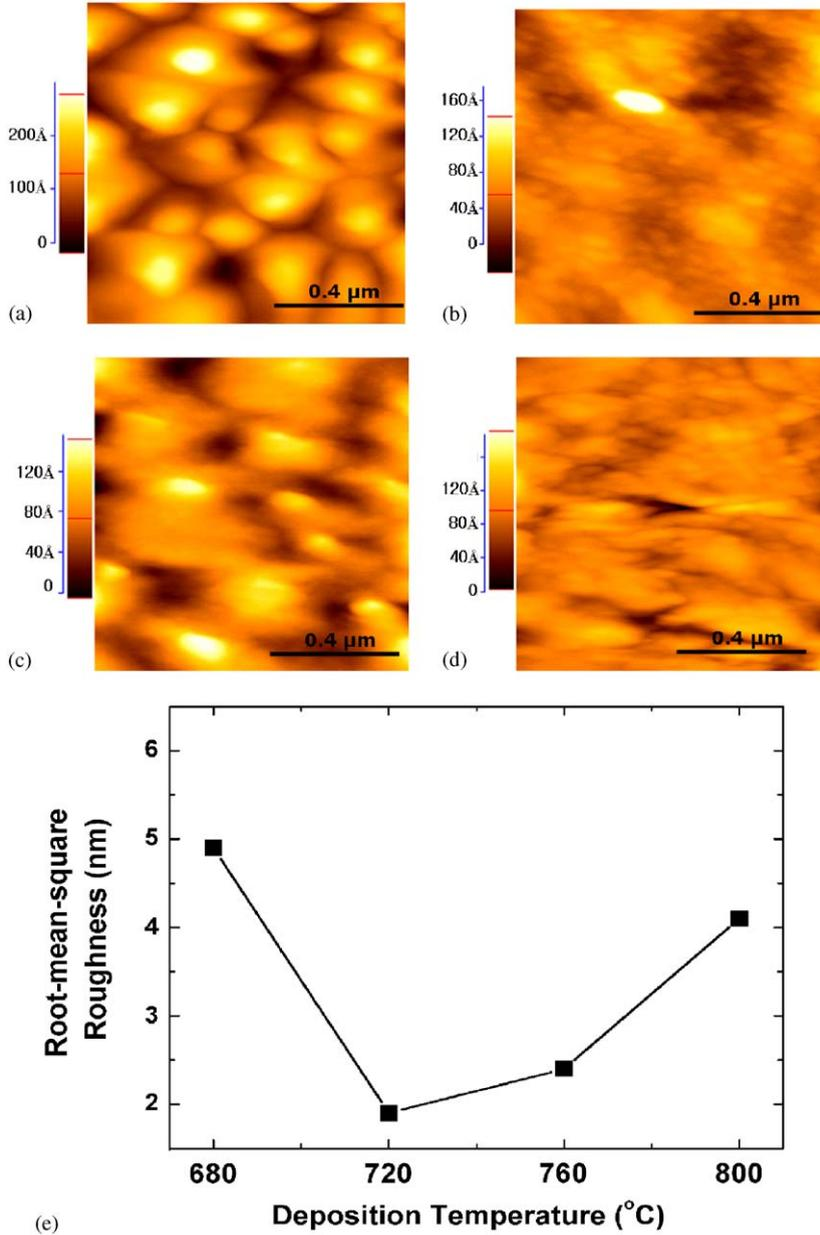
Fig. 2. AFM images of the ZnO films deposited at (a) 680 °C (b) 720 °C (c) 760 °C, and (d) 800 °C, respectively. (e) Calculated root-mean-square roughness of the ZnO films.
