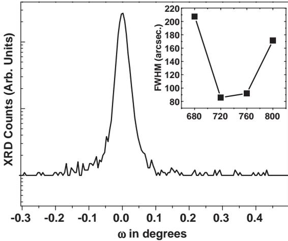
Fig. 3. XRD  $\omega$ -rocking curves of the ZnO (0002) films deposited with on  $\text{Al}_2\text{O}_3$  (0001) substrates with different growth temperatures.
