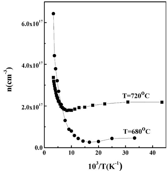
Fig. 1. Carrier concentration as a function of inverse temperature for the ZnO films grown at 680 °C (●, ZN-1) and 720 °C (■, ZN-2).
