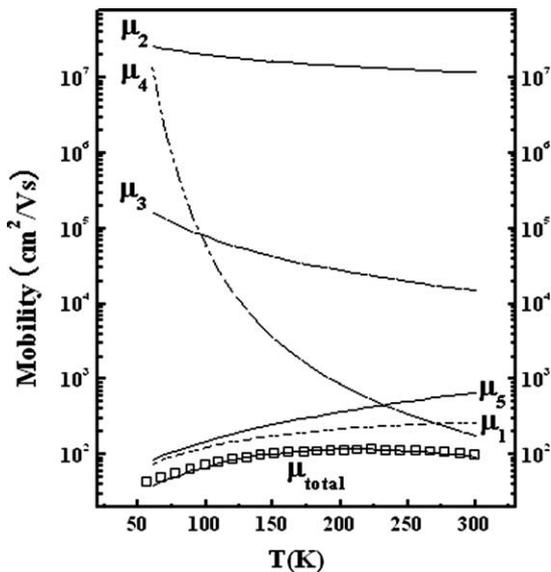
Fig. 3. Experimental (■) and calculated (solid line) Hall mobility as a function of temperature in ZnO thin films deposited at 720 °C (ZN-2) by plasma-assisted MBE. Different components of the mobility are also shown.
