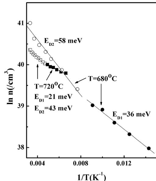
Fig. 2. Logarithmic Hall concentration as a function of inverse temperature for the ZnO films grown at 680 °C (●, ZN-1) and 720 °C (■, ZN-2).
