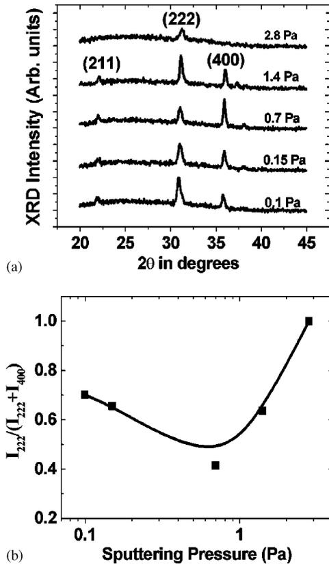
Fig. 6. Change of: (a) XRD profiles and (b)  $(I_{(222)})/(I_{(222)}+I_{(400)})$  depending upon sputtering pressure.
