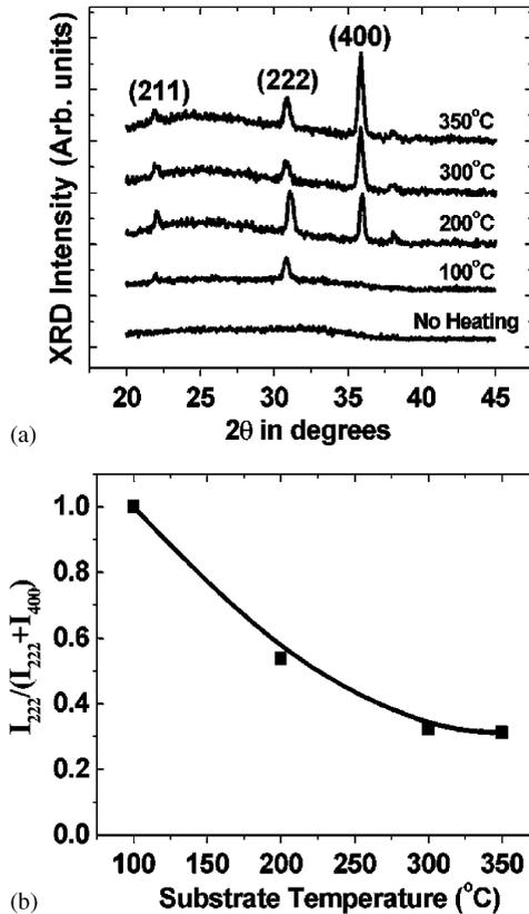
Fig. 8. Change of: (a) XRD profiles and (b)  $(I_{(222)})/(I_{(222)}+I_{(400)})$  depending upon substrate temperature.
