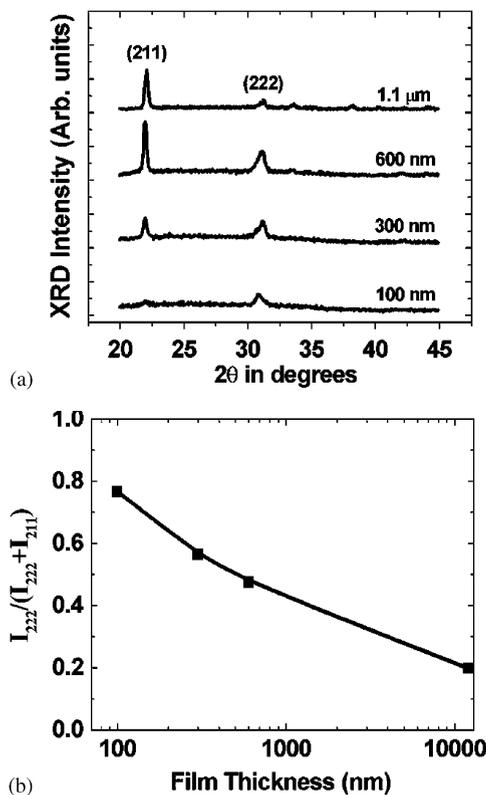
Fig. 3. Change of: (a) XRD profiles and (b)  $(I_{(222)})/(I_{(222)}+I_{(400)})$  depending upon film thickness (oxygen flow of 6 sccm).
