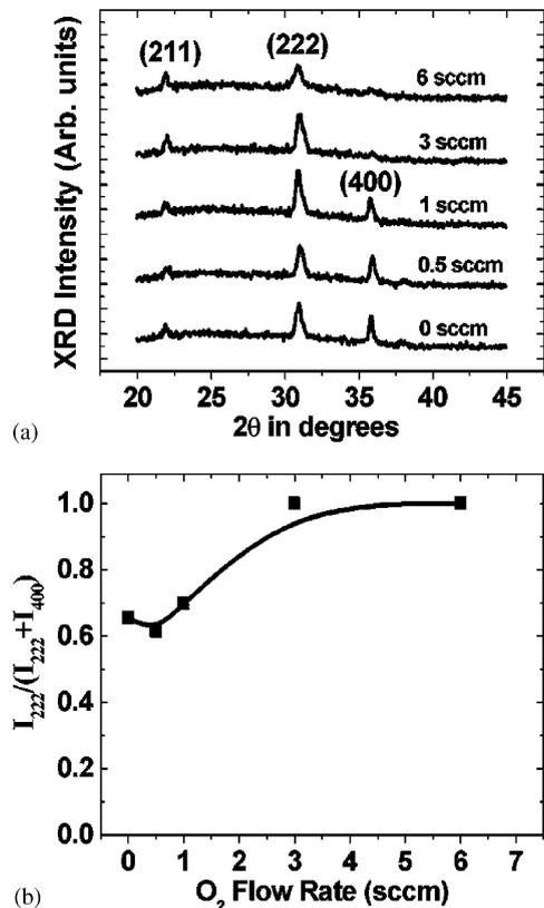
Fig. 5. Change of: (a) XRD profiles and (b) ( $I_{(222)}/(I_{(222)}+I_{(400)})$ ) depending upon oxygen flow rate.
