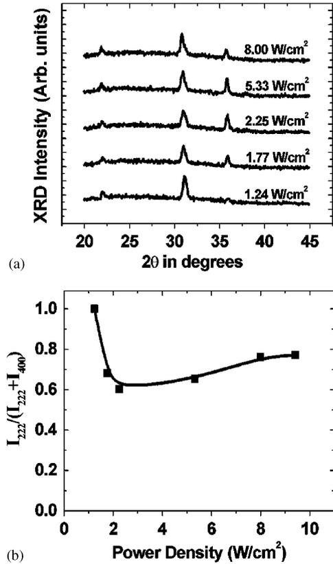
Fig. 7. Change of: (a) XRD profiles and (b)  $(I_{(222)})/(I_{(222)}+I_{(400)})$  depending upon sputtering power.
