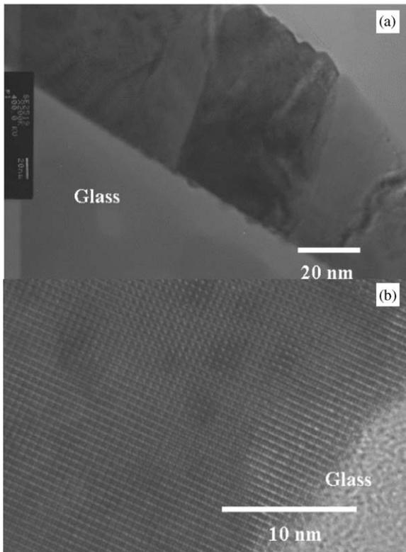
Fig. 1. Cross-sectional TEM images of ITO films deposited on glass substrates.
