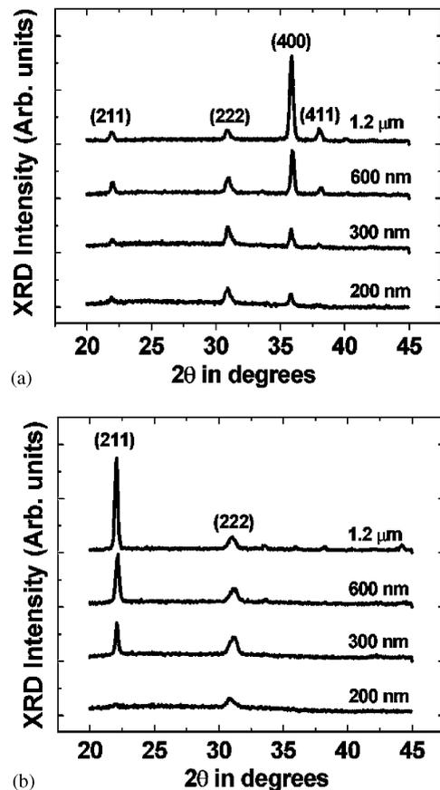
Fig. 4. Change of XRD profiles of the samples prepared with mixed conditions: (a) initially no oxygen, later 6 sccm and (b) initially oxygen flow of 6 sccm, later no oxygen.
