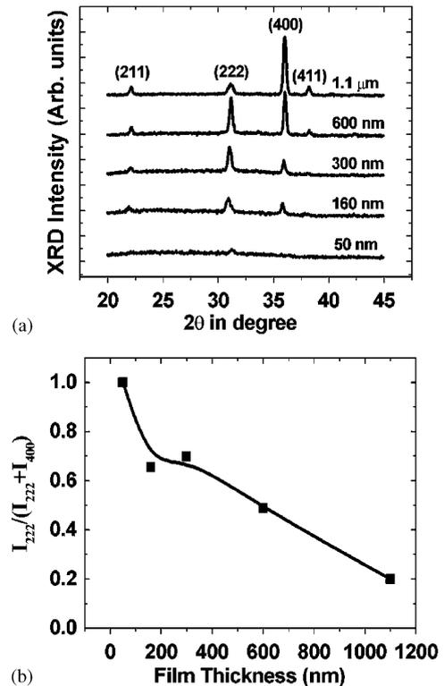
Fig. 2. Change of: (a) XRD profiles and (b) ( $I_{(222)}/(I_{(222)}+I_{(400)})$ ) depending upon film thickness (no oxygen condition).
