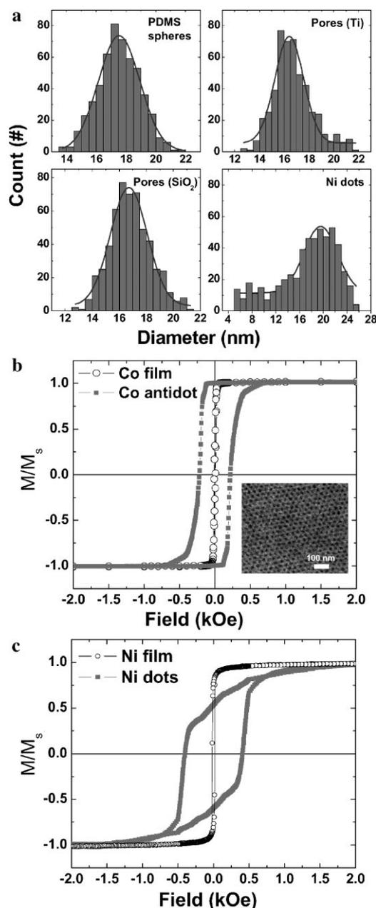
**Figure 4.** a) Size histograms of PDMS dots, pores formed in Ti and SiO<sub>2</sub>, and Ni dots. The magnetic hysteresis loops of b) a Co antidot pattern and c) Ni dots, compared with the hysteresis of unpatterned Ni and Co thin films.
