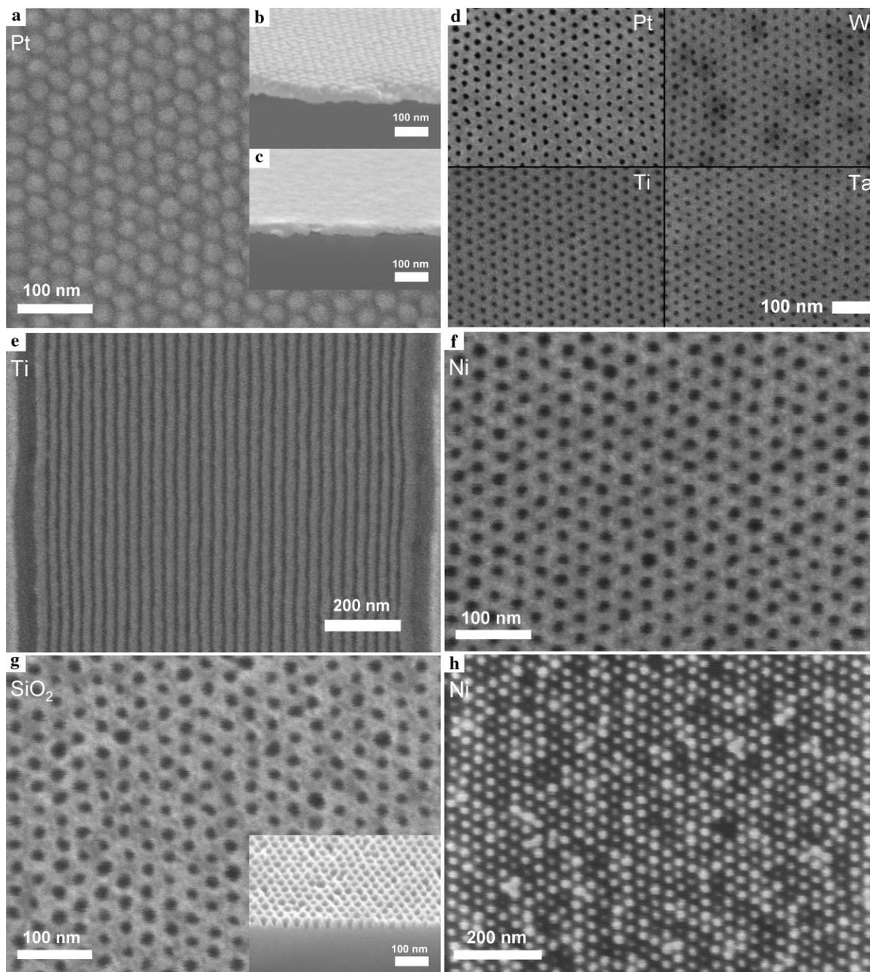
**Figure 3.** SEM images of a and b), a Pt thin film sputter-deposited on oxidized PDMS spheres, c) smoothed surface of the Pt after a high-power  $\text{CF}_4$  plasma treatment, d) various metallic thin films with nanopores after the selective removal of the PDMS template, e) Ti nanowire patterns, f) a nanoporous Ni film on  $\text{SiO}_2$ , g) patterned  $\text{SiO}_2$  via  $\text{CF}_4$  reactive ion etching and Ni wet-etching, and h) a Ni dot array.
