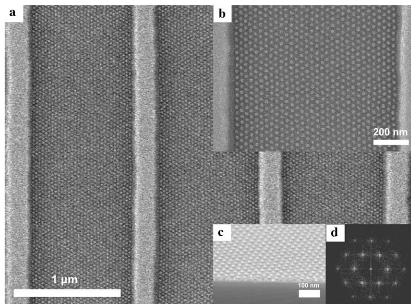
**Figure 2.** a–c) SEM images of self-assembled block-copolymer patterns after reactive ion etching. The oxygen plasma selectively removes the PS matrix block and oxidizes the PDMS spheres. d) The fast Fourier transform (FFT) of (b).
