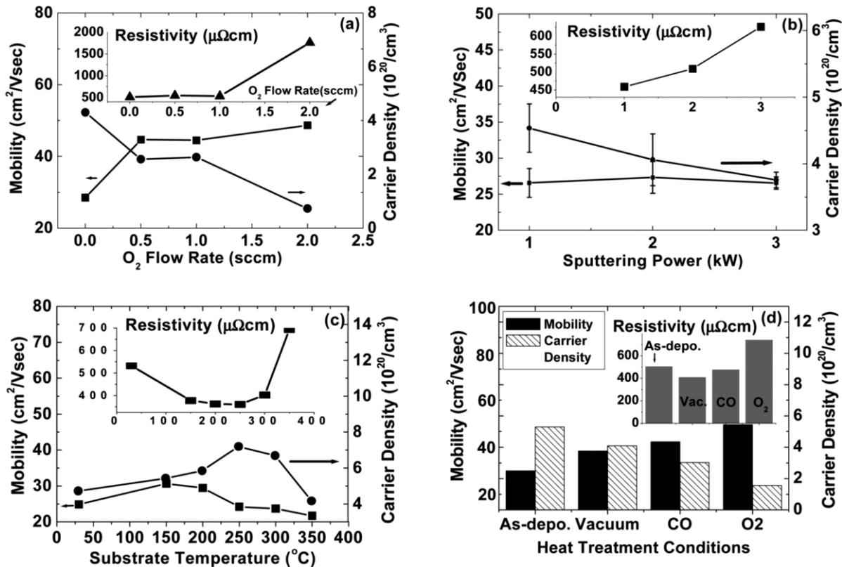
Fig. 5. Variations of the resistivity, the carrier concentration and the mobility of IZO films depending upon (a) oxygen flow rate, (b) sputtering power, (c) substrate temperature and (d) heat treatment atmosphere.
