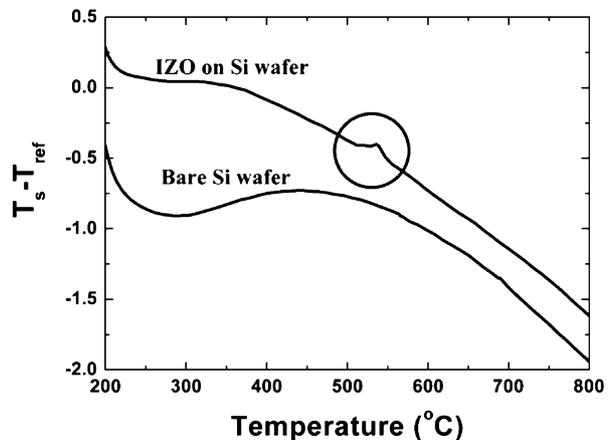
Fig. 2. DTA curves of a bare Si wafer and an IZO thin film deposited on Si wafer.
