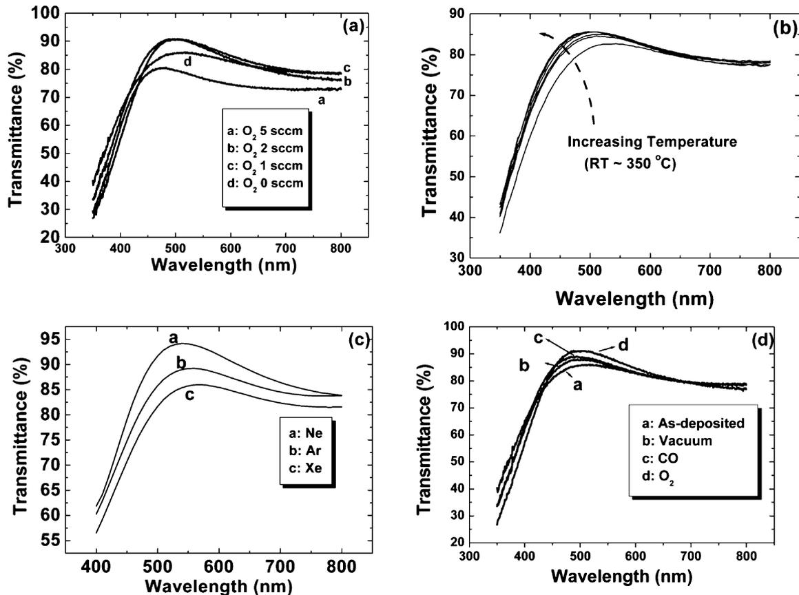
Fig. 7. Transmittance curves depending upon (a) oxygen flow rate, (b) deposition temperature, (c) sputtering gas and (d) heat treatment atmosphere.
