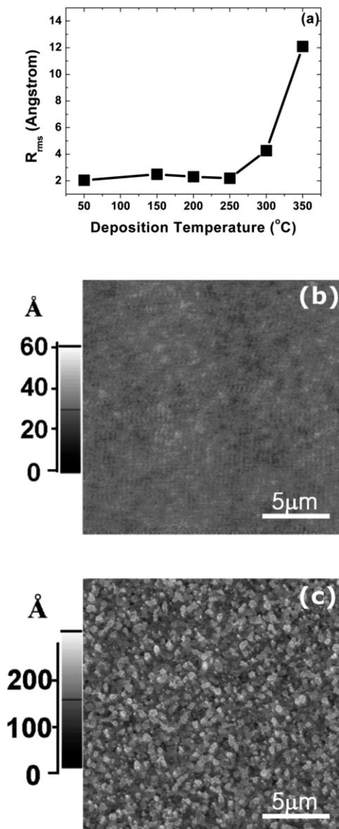
Fig. 3. (a) Surface roughness change depending upon deposition temperature and three-dimensional images of IZO films deposited at (b) RT and (c) 350 °C.
