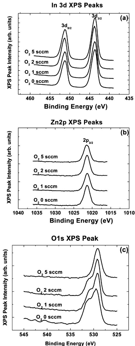
Fig. 4. Changes of (a) In3d, (b) Zn2p and (c) O1s XPS spectra of IZO thin films as a function of oxygen flow rate.
