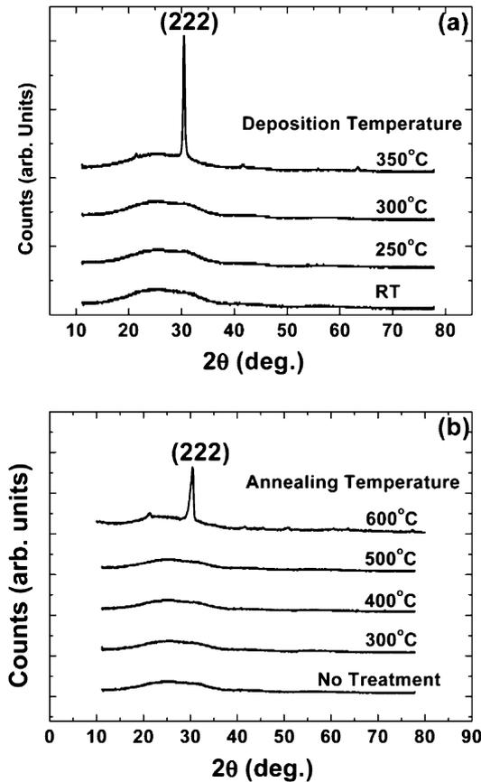
Fig. 1. XRD spectra taken from IZO thin films deposited on glass substrates depending upon (a) deposition temperature and (b) heat treatment temperature.
