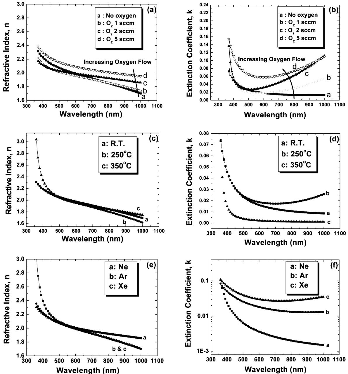
Fig. 6. Variations of indices of refraction and extinction coefficients depending upon (a), (b) oxygen flow rate, (c), (d) deposition temperature and (e), (f) sputtering gas, respectively.
