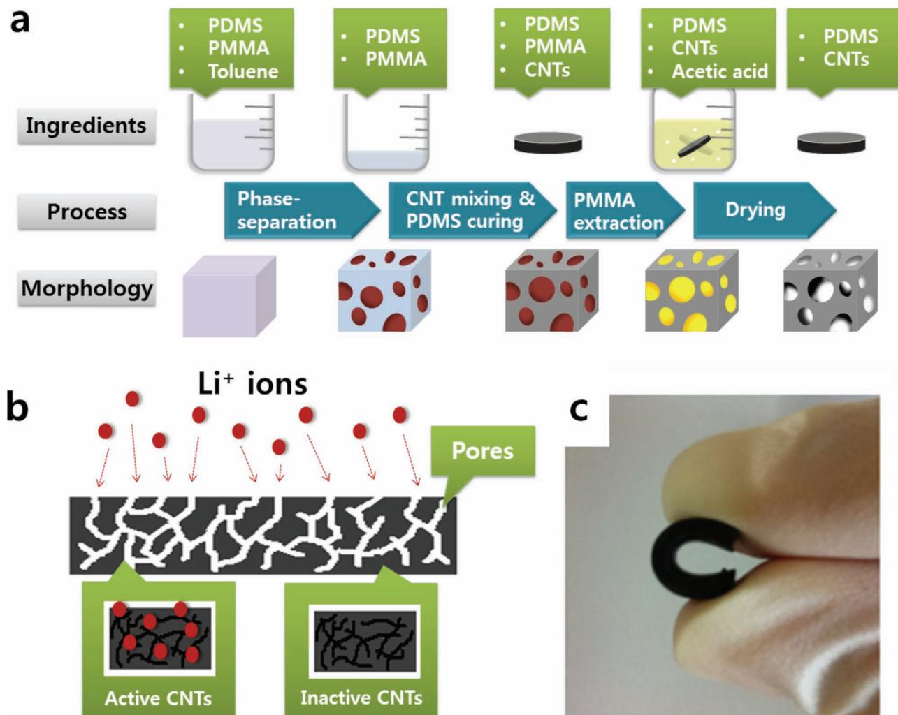
**Figure 1.** a) The procedure to fabricate the porous PDMS–CNT nanocomposites. b) Schematic representation of the PDMS–CNT nanocomposites with porous channels for the effective penetration of electrolytes and lithium ions. c) An example of porous PDMS–CNT nanocomposites demonstrating high mechanical flexibility.
