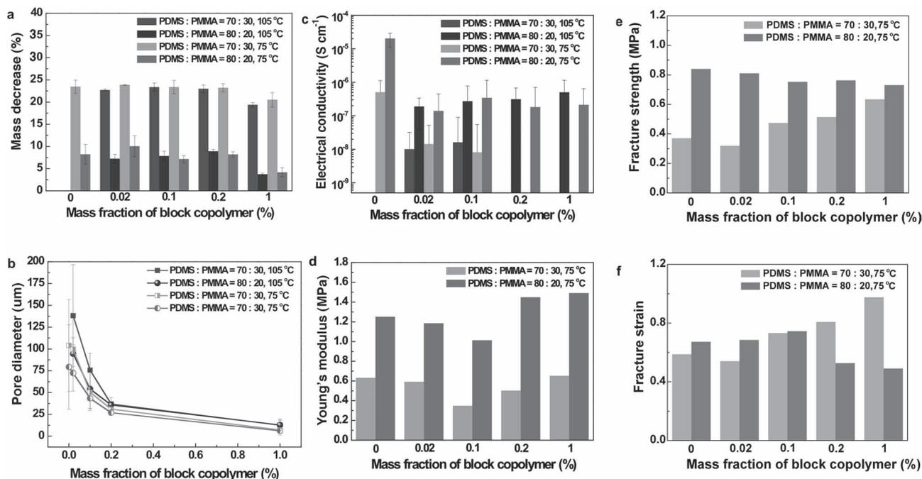
**Figure 3.** Statistical measurement data of a) mass decrease after the removal of the PMMA by an acetic acid treatment, b) diameter of the pores, c) electrical conductivity, d) Young's modulus, e) fracture strength and f) fracture strain depending on the portion of PMMA and PDMS-*b*-PMMA and on the drying temperature. Missing data in (b,c) are due to macroscopic phase separation or because the conductivity was too low.
