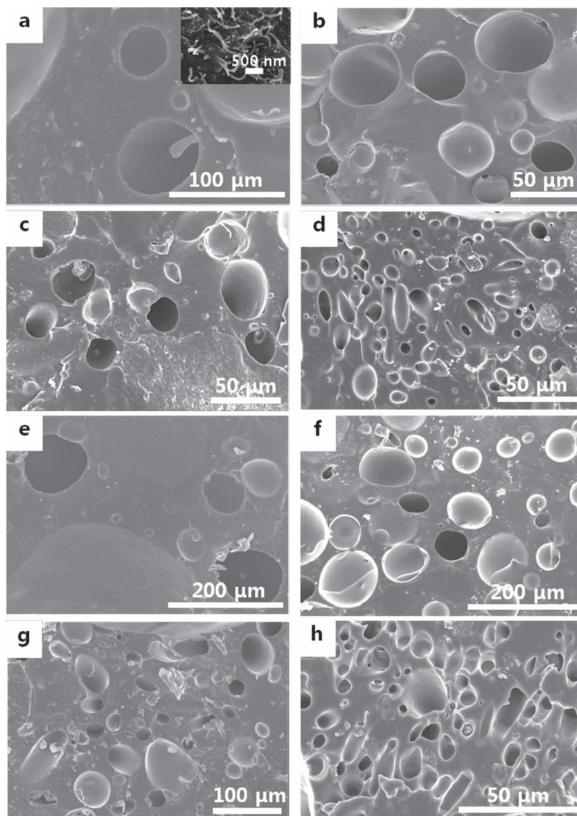
**Figure 2.** SEM images of the porous morphologies of the samples prepared with different fractions of PMMA and the block copolymer in the initial mixture. The weight fraction of the embedded CNTs and the solvent drying temperature were fixed at 5% and 75 °C, respectively. The weight fractions of the PMMA were a–d) 20% and e–h) 30%. The fractions of the PDMS-*b*-PMMA block copolymers were a,e) 0.02, b,f) 0.1, c,g) 0.2%, and d,h) 1%. The inset in (a) shows CNTs loaded in the nanocomposite.
