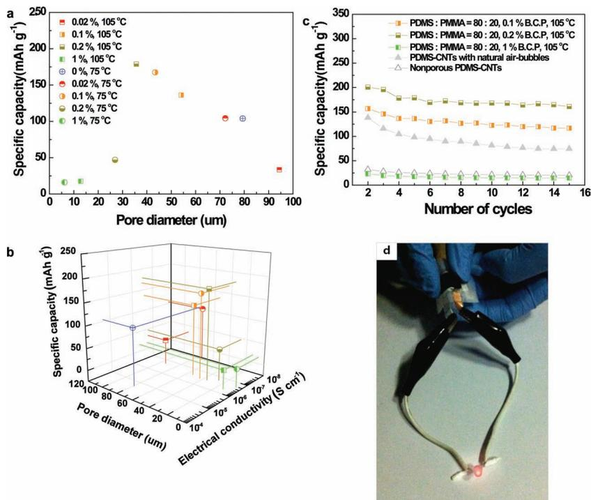
**Figure 4.** a) Capacity per mass of active material of the 80:20 samples depending on the pore size. b) 3D representation of the capacity of the 80:20 samples as a function of pore size and of the electrical conductivity. c) The cycle retention of some 80:20 samples during the first 15 cycles. In (a,b), the values after the fifth cycle are presented. d) A flexible lithium-ion battery full cell fabricated with the porous PDMS-CNT nanocomposites as the anode and LiCoO<sub>2</sub> as the cathode.
