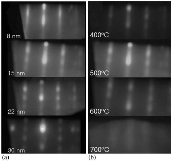
Fig. 1.  $\langle 1\bar{2}10 \rangle$  RHEED patterns of the ZnO buffer layers after thermal-treatment for 30 min at 800°C. The thin films were prepared with varying: (a) thickness and (b) deposition temperature.
