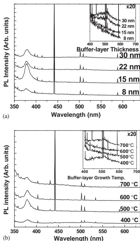
Fig. 3. PL spectra of the ZnO films deposited with: (a) the buffer-layer thickness; and (b) the different buffer-layer deposition temperatures.
