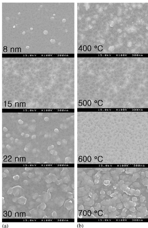
Fig. 2. SEM images of the 100 nm thick ZnO films deposited with (a) the buffer-layer thickness and (b) the different buffer-layer deposition temperature.
