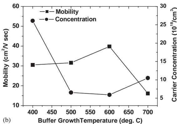
Fig. 5. Hall measurement results of the ZnO films deposited with: (a) the buffer-layer thickness; and (b) the different buffer-layer deposition temperatures.
