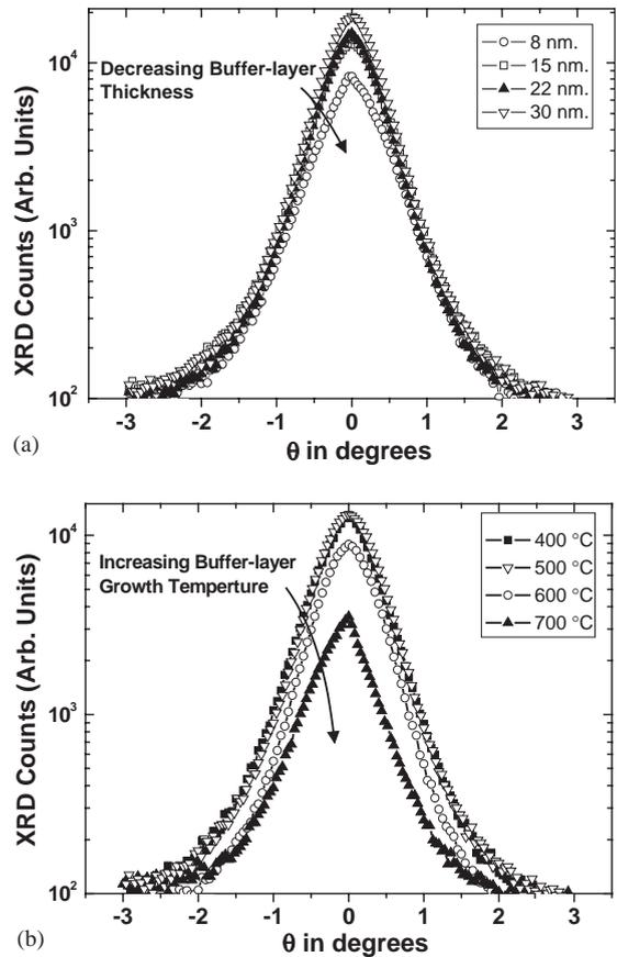
Fig. 4. XRD  $\theta$ -rocking curves of the ZnO (0002) films deposited with: (a) the buffer-layer thickness; and (b) the different buffer-layer deposition temperatures.
